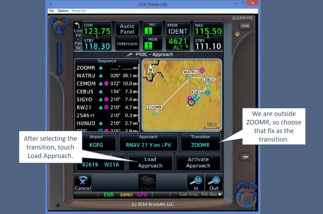
Loading an approach simply adds all of the fixes for the approach to the Active Flight Plan, below the destination airport.
